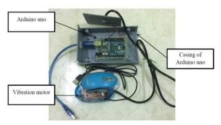
Fig. 2 Mouse with a DC motor as a vibrator
