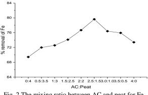
Fig. 2 The mixing ratio between AC and peat for Fe removal
