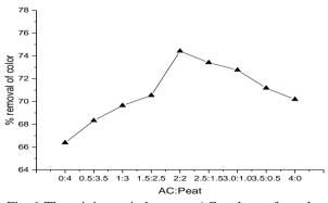
Fig. 1 The mixing ratio between AC and peat for color removal
