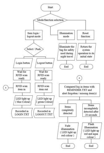
Fig. 5 Block diagram of the RFID-based Interactive Log Bag operating system
