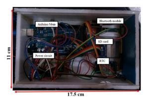
Fig. 3 The built-in circuit for the RFID-based item detection and logging system
