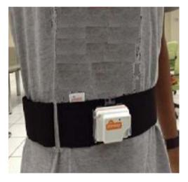
Fig. 3 Accelerometer sensor worn on the subject's waist
