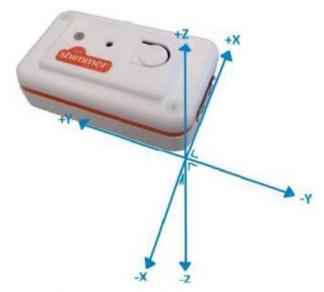
Fig. 2 Shimmer three-axial wireless-based accelerometer.
