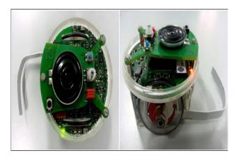
Fig. 3.2 The top view and the side view of the L-shape object gripper with a dimension of  $4\text{cm} \times 4\text{cm}$  attached at the back of the E-puck robot.
