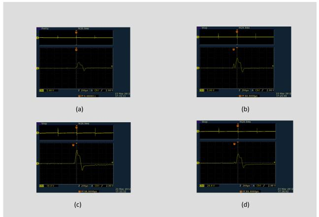
Figure 5 is about the signal change due to the changes of the input current from the movement of knee joint after pasted by the FES electrode; (a) is about 10 mA of input current, (b) about 30mA input current, (c) 60 mA input current and lastly (d) about 90 mA input current.
