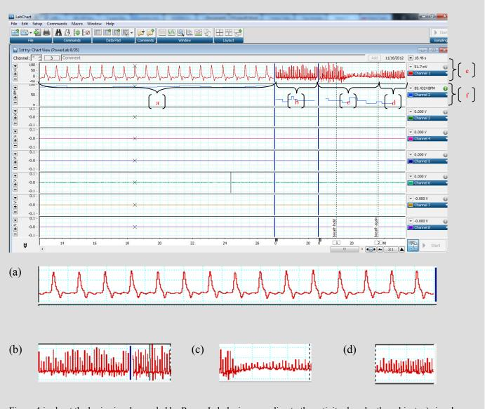
Figure 4 is about the brain signal recorded by Power Lab device according to the activity done by the subject: a) signal in zoom in mode b) signal for normal breathing c) signal when holding breath d) signal when breathing again e) raw data rate f) calculation data rate
