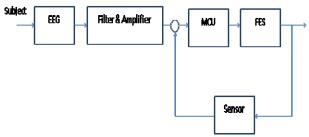
Figure 3: BCI-FES Control Scheme System
