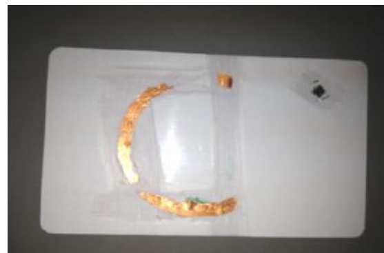
Figure 4: RFID Tag Antennas from Copper Etched
