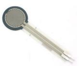
Fig. 2 Force sensitive resistor (FSR) [17]
