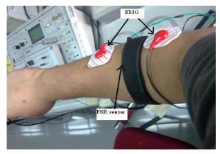
Fig. 7 Location of EMG and FSR targeted medial extensor carpi radialis on the lower arm.
