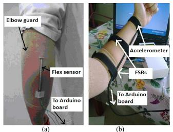
Fig. 15 (a) Elbow guard attached with flex sensor, (b) Location of the other sensors.
