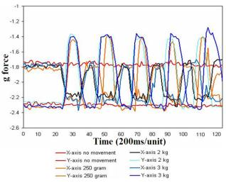
Fig. 12 Voltage output from accelerometer based on different weight during object lifting activity.
