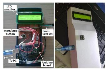
Fig. 16 Hardware setup of the main unit for the monitoring device.(a) actual main unit circuitry (b) main unit with custom built box.
