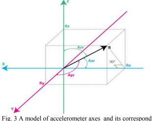
Fig. 3 A model of accelerometer axes and its correspond force vectors (Rx,Ry,Rz) and angles (Axr, Axy and Axz)[16].
