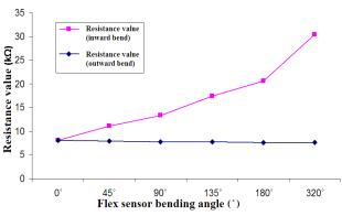
Fig. 5 Resistance value against flex sensor bending angle.
