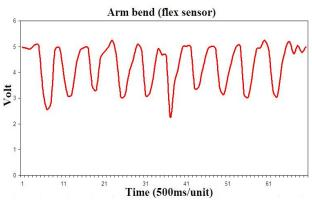
Fig. 6 Flex sensor voltage value due to arm bending movement.
