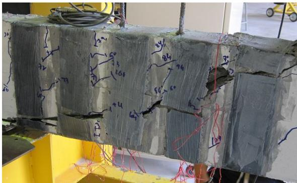
Fig. 6: Cracking and failure pattern of beam C2.5-UA-V2
