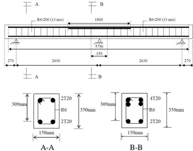
Fig. 1: Reinforcement and cross section details
