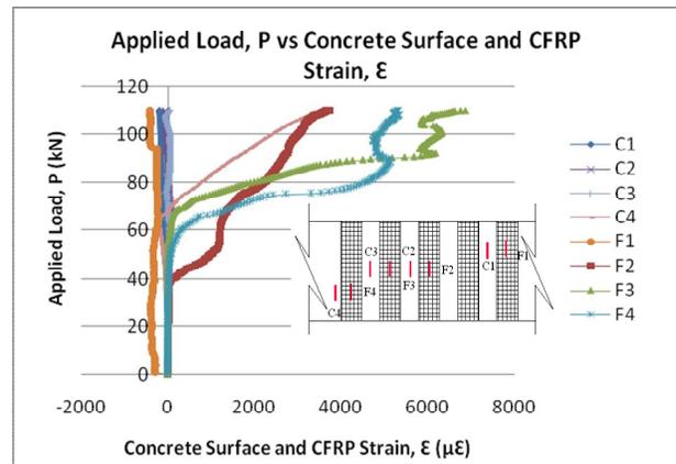
Fig. 12: Graph of Applied Load vs Concrete Surface and CFRP Strain for C2.5-UA-V2
