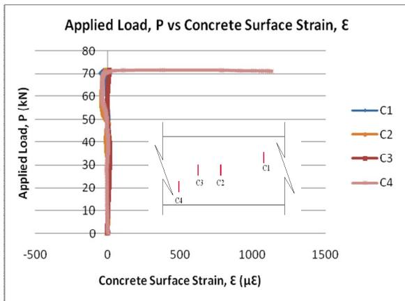
Fig. 9: Graph of Applied Load vs Concrete Surface and CFRP Strain for C2.5-C
