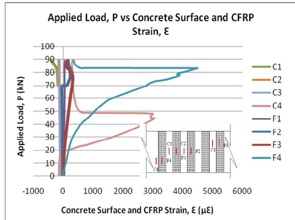
Fig. 11: Graph of Applied Load vs Concrete Surface and CFRP Strain for C2.5-U-V
