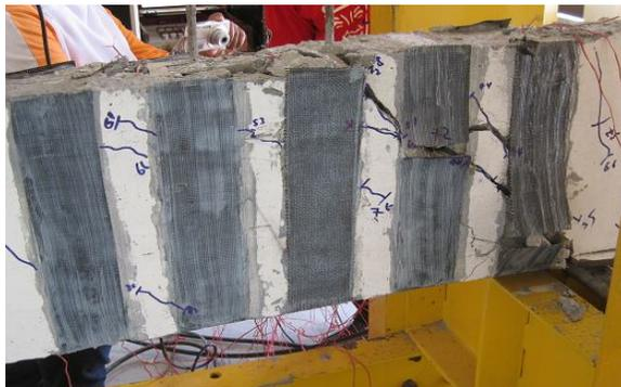
Fig. 5: Cracking and failure pattern of beam C2.5-U-V
