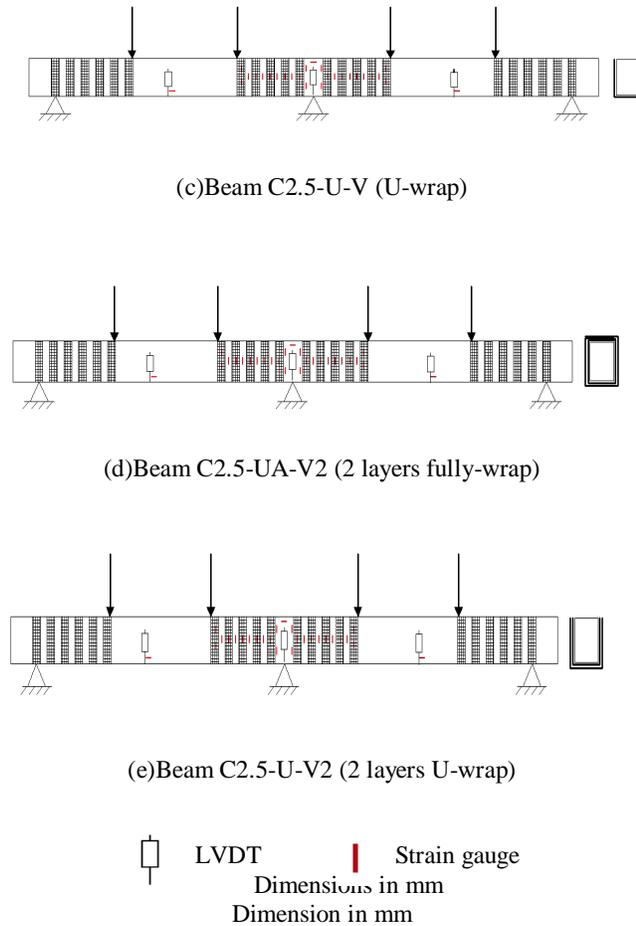
Fig. 2: Test set-up and strengthening schemes
