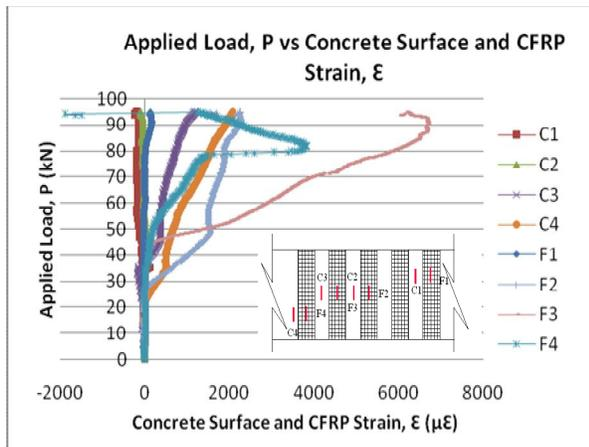
Fig. 10: Graph of Applied Load vs Concrete Surface and CFRP Strain for C2.5-UA-V
