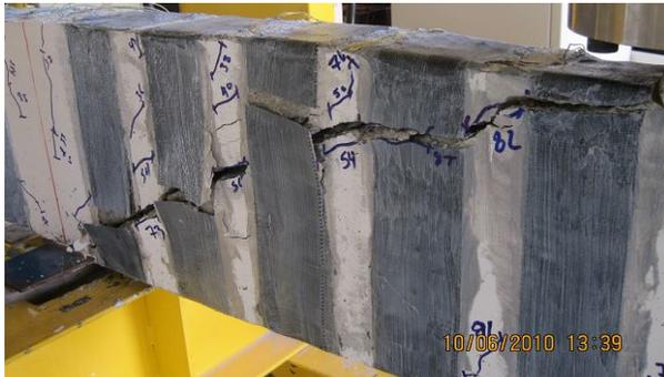
Fig. 4: Cracking and failure pattern of beam C2.5-UA-V
