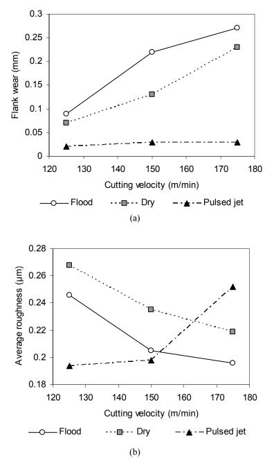
Fig. 2 Effect of cutting velocity on (a) flank wear and (b) surface roughness in slot milling test
