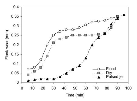
Fig. 6 Flank wear progress for slot milling
