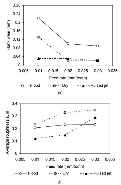
Fig. 3 Effect of feed rate on (a) flank wear and (b) surface roughness in slot milling test
