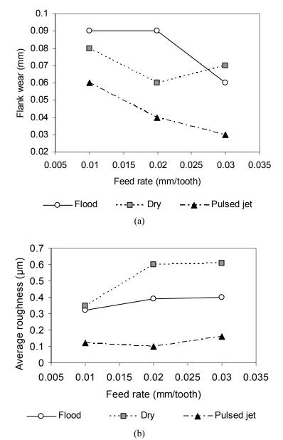
Fig. 5 Effect of feed rate on (a) flank wear and (b) surface roughness in down milling test
