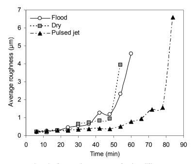
Fig. 7 Surface roughness progress for slot milling
