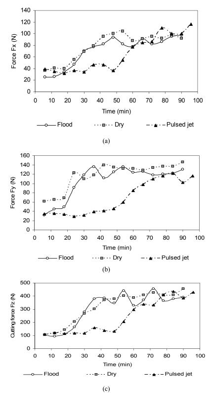
Fig. 5 Cutting force progress for slot milling (a)  $F_x$ , (b)  $F_y$  and (c)  $F_z$
