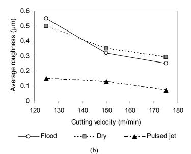
Fig. 4 Effect of cutting velocity on (a) flank wear and (b) surface roughness in down milling test
