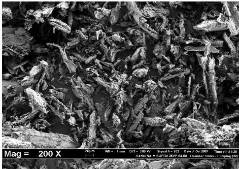
Fig. 4 SEM micrograph of kenaf powder.
