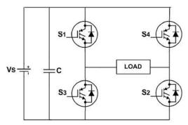
Fig. 1 Single phase Full-Bridge Inverter
