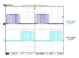
Fig. 11 Output signal for S1S2 and S3S4 with modulation index= 0.75
