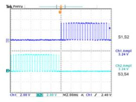
Fig. 7 Output signal for modulation index 0.75
