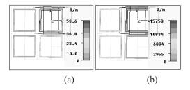
Fig. 2.4: (a) Surface current distribution (b) Efield intensity on the patch elements at theta = 75 degree
