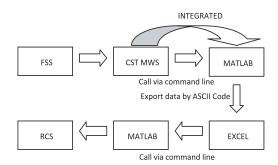
Fig. 2.3 Flow of the FSS array study on the RCS Reduction.
