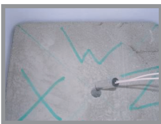
Fig. 2 Detonator charge insertion
