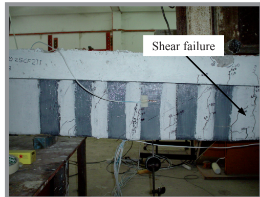
Fig. 2(c) Flexural failure pattern of initially CFRP strengthened beam TT1-1I
