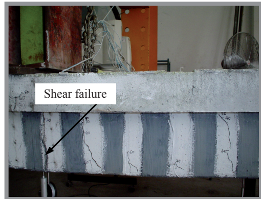
Fig. 2(g) Flexural failure pattern of precracked repaired beam TS2-1
