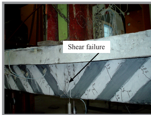
Fig. 2(e) Flexural failure pattern of precracked repaired beam TT2-2
