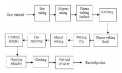
Fig.6 A schematic of workstations in an assembling production line
