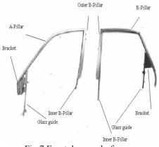
Fig.7 Front door-sash for car
