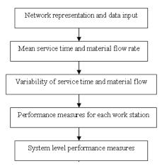
Fig. 2 Procedure to calculate performance measures on spreadsheet model
