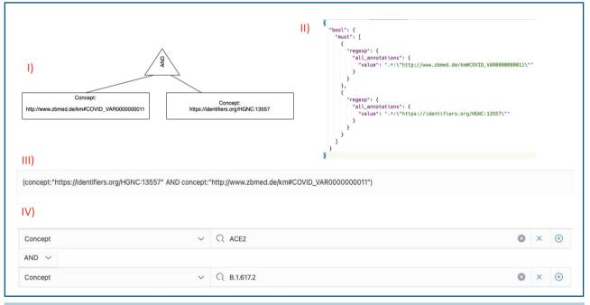
**Fig. 3.** A Search Query shown in AST (I), ElasticSearch DSL(II), preVIEW DSL (III) and Query Builder Component (IV).
