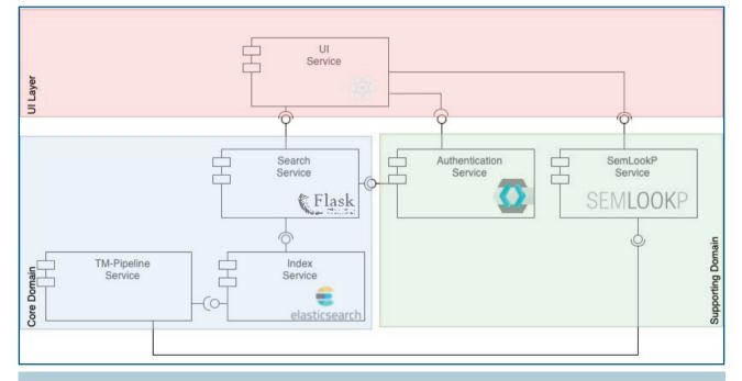
Fig. 1. Component diagram of the preVIEW System.
