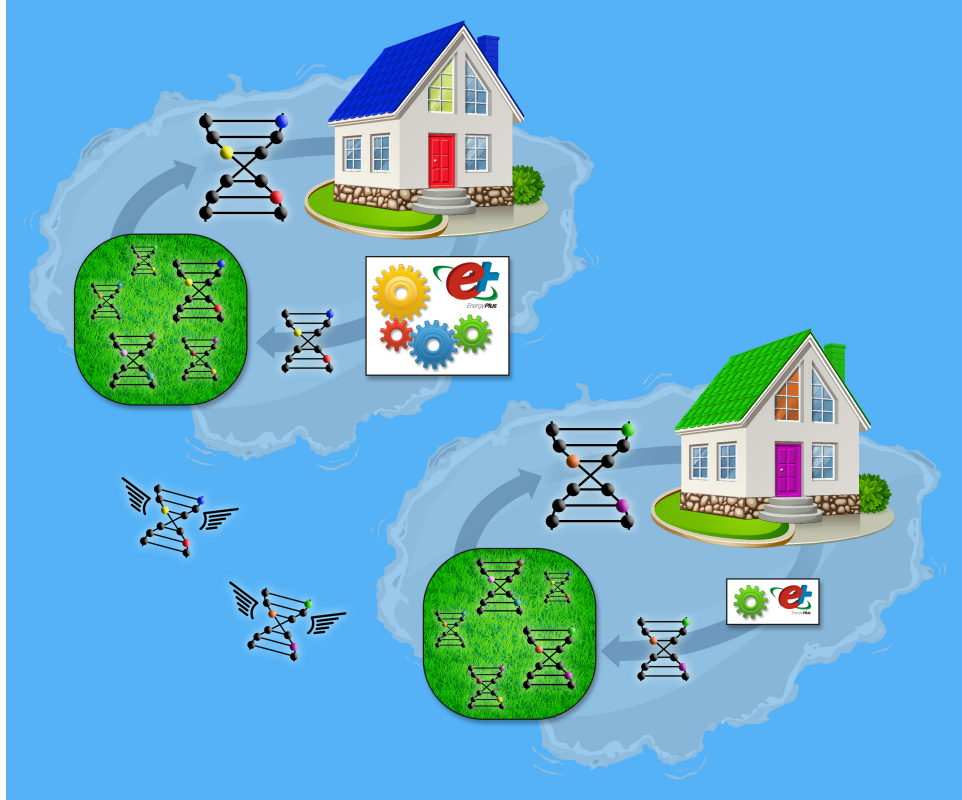
Figure 4: In this illustration, the upper-left island uses the full year schedule (represented by the large EnergyPlus “black box”), and the other island at the lower-right uses the abbreviated schedule. Candidate solutions migrating periodically between the islands are represented as winged candidate solutions en route . When these candidate solutions arrive at their destination islands, they must be re-evaluated to determine their appropriate size.
