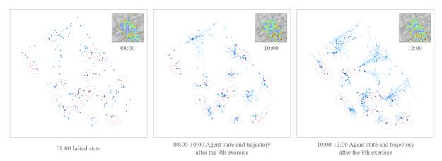
Since each picture performs 10 operations, the agent moves 10 times. At the same time as the tenth operation, recalculate the attraction point based on the new heat map (the next moment). The agent always moves towards the nearby attraction point (refer to the heat map at 08:00 and 10:00 on August 21, 2020)
