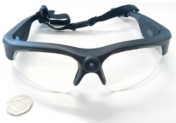
Figure 1. The SunnyCam Sport used in this study next to a 20 pence coin (£0.20) for scale (coin diameter: 2.14 cm).
