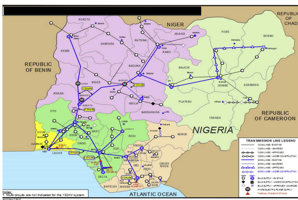
Figure 6. National electricity transmission grid of Nigeria (Source: [61]).
