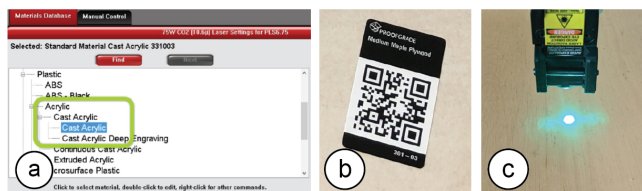
Figure 2: Existing material identification approaches: (a) Manually selecting from a database (e.g., ULS [50]) or (b) scanning QR code stickers on sheets (Glowforge). (c) SensiCut uses speckle sensing to identify the material based on its surface structure without the need for additional tags.
