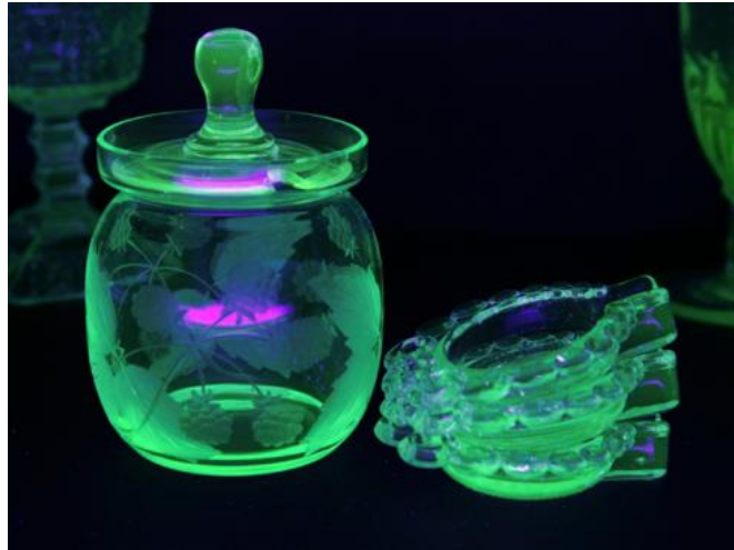
Figure 2 - Glass made with Manganese Dioxide under a blacklight. (15)
