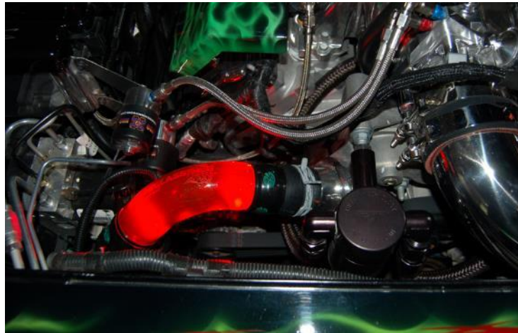
Figure 13 - Glass being used within Pipe coolant systems in a motor vehicle. (80)
