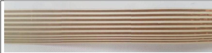
Figure 90 Flexible ribbon cable with multiple 1mm and 0.5mm tracks
