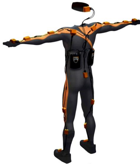
Figure 17 Suit designed for quick use and convenient placement of the Xsens MVN sensors [59]
