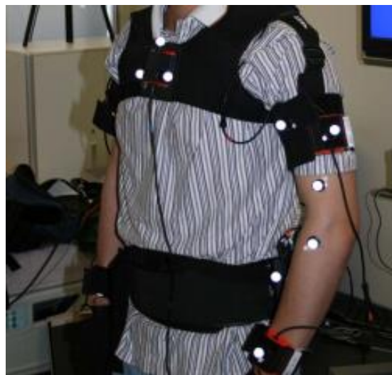
Figure 16 Configuration of MTx inertial sensors and optical markers for human upper limb motion estimation assessment procedure [54]
