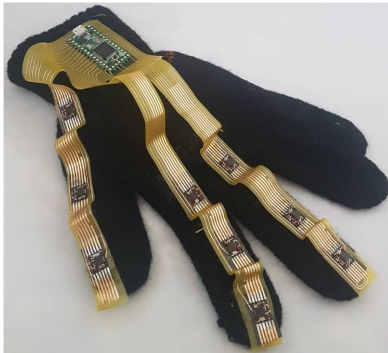
Figure 98 Glove with three fingers setup for motion capturing, using 'striped' module and flexible ribbon cable connectors. Teensy 3.2 microprocessor used at the wrist of the glove
