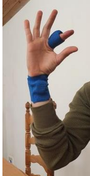
Figure 36 Photo of the two setups used for the Parkinson's dataset. An MMR device is strapped to the wrist and around the base of the index finger using cohesive tape.
