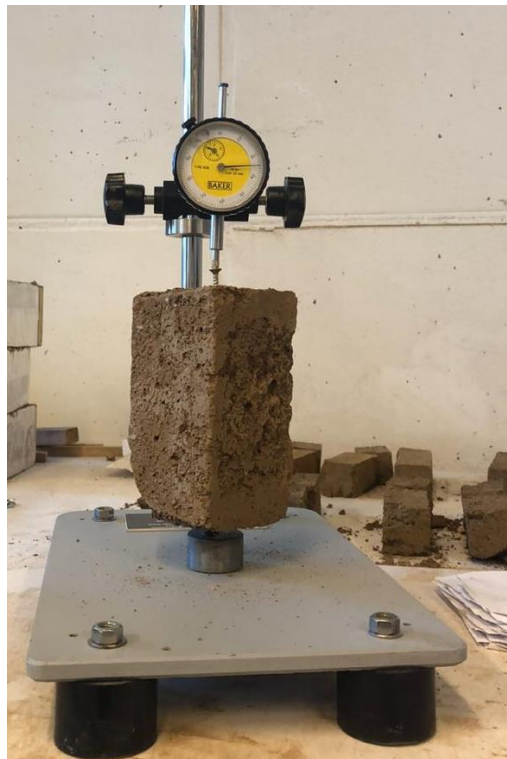
230 Figure 6: Length change testing apparatus and specimen using 75 by 75 by 140 mm samples
