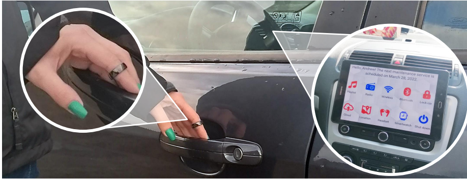
Fig. 2. Interaction with the smart vehicle in the personal zone: an NFC ring receives data from the vehicle when in contact with an active NFC component from the vehicle.
