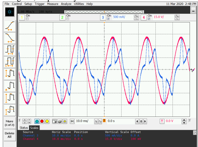
Fig. 13 The input current (blue) and power supply voltage (red) without compensation at 50Hz
