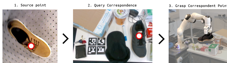
Figure 1: Correspondence (red circle) produced by our DON+Soft method used for robot grasping.
