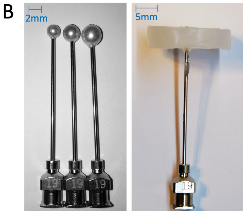
Figure 2-1 Ball-tip nozzles Structure
