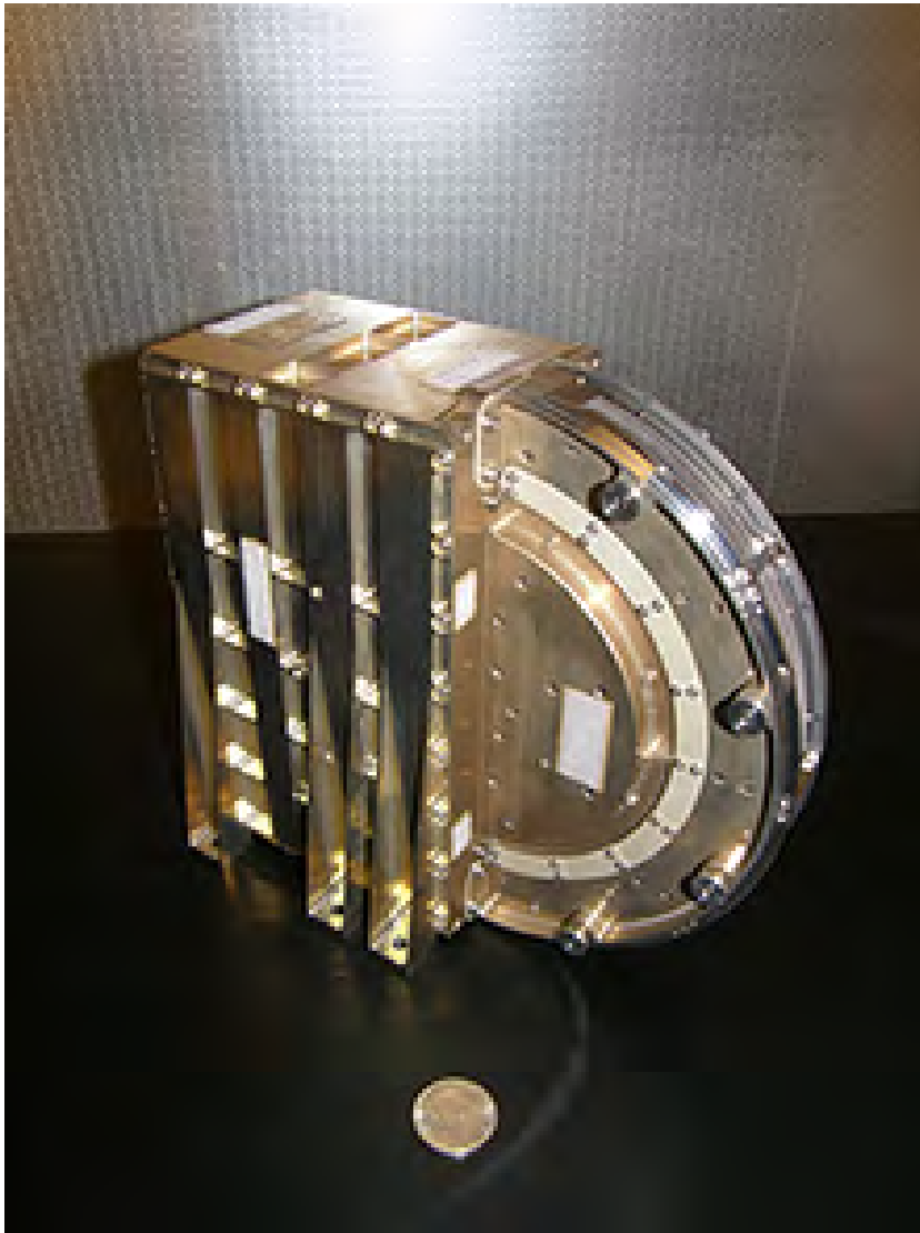
Fig. 73 ENA flight model. The sensor is wrapped by MLI, when ENA is installed in the spacecraft.
