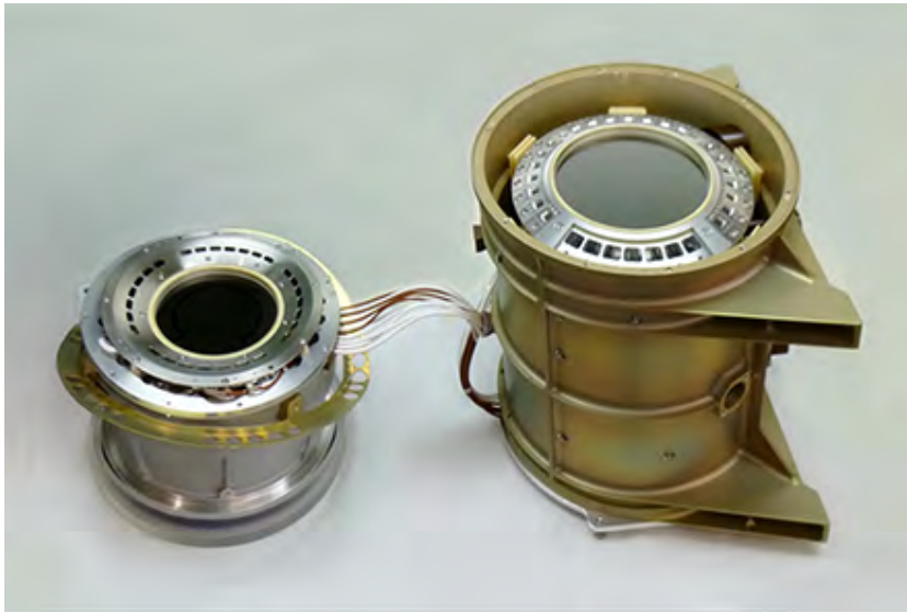
Fig. 42 Energy analyzer (left, viewed from the back), and TOF chamber (right, view from top).
