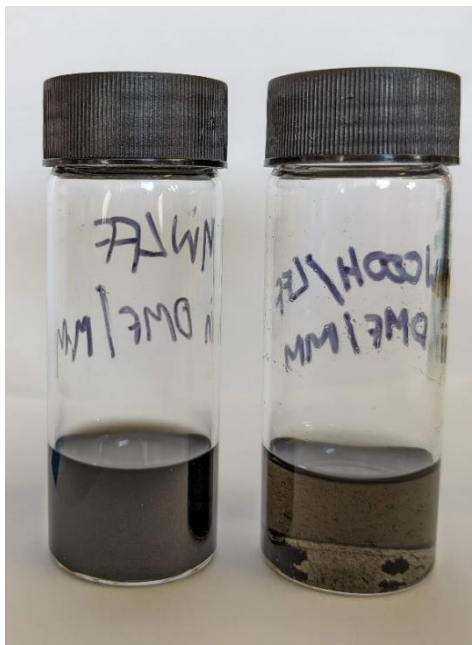
Figure 4.3 Dispersions (in a DMF/ N-methylmorpholine mixed solvent) of MWLFF complex (left) and a mixture of MWCNT-COOH and L-diphenylalanine (right) after a one hour resting period post dispersion
