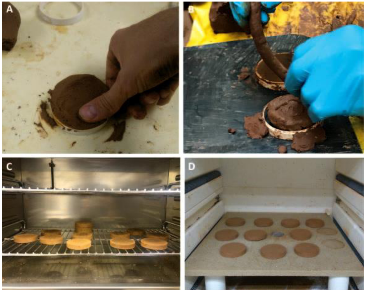
Figure A7.15: Manufacturing of ceramic discs: (a) pressed/pinched specimens, (b) coiled specimens, (c) drying in oven, and (d) firing of specimens in pottery kiln.
