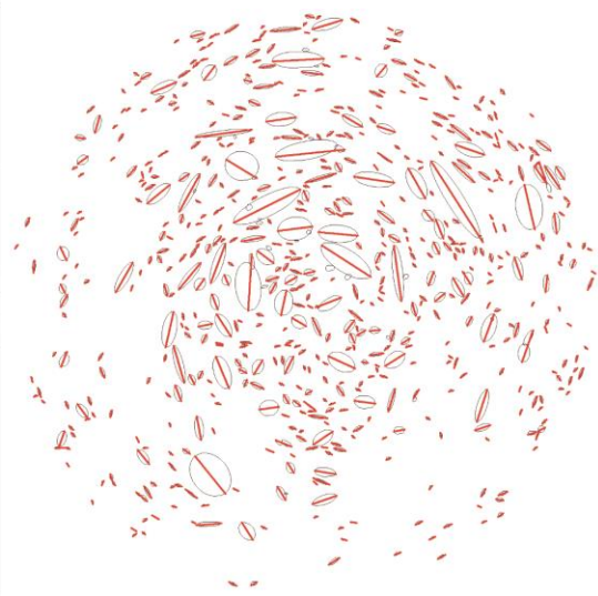
Figure A7.18: X-ray radiographs of dung-tempered experimental discs (left) and processed images showing orientation of fibres (right). Red lines indicate the longest axis of particles and pores.
