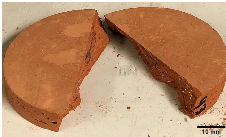
Figure 9.12: Remaining chaff fibres potentially acting as crack bridges.
