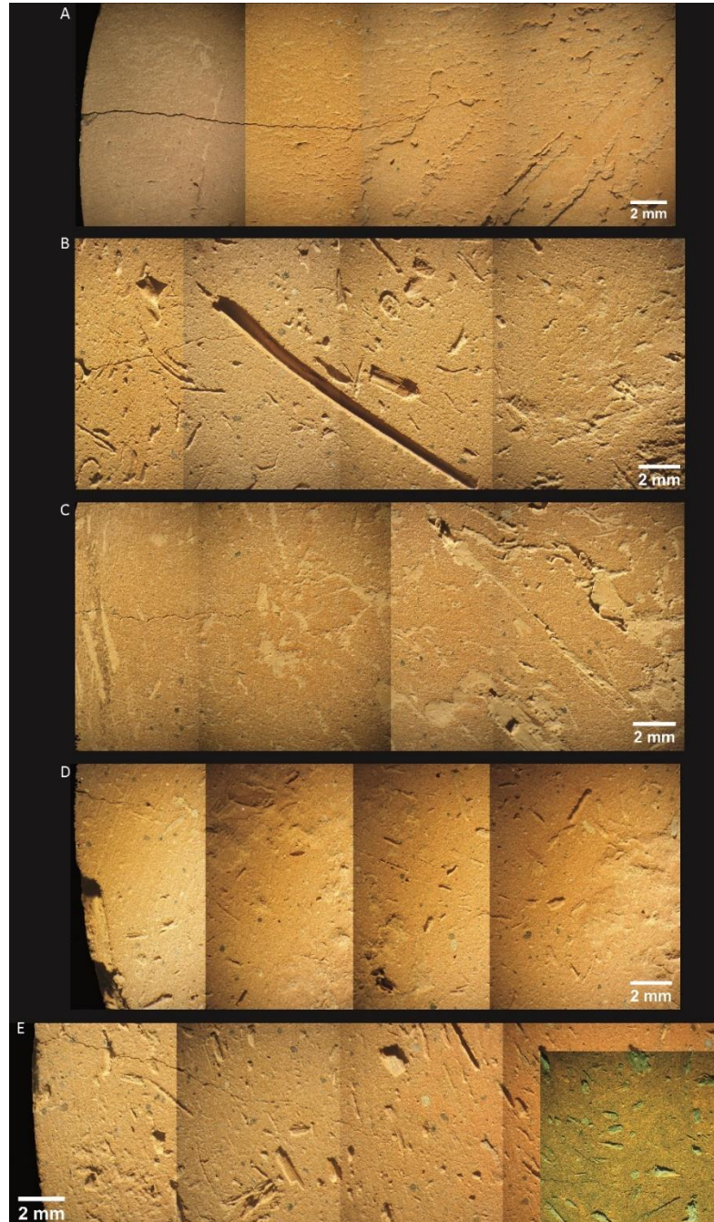
Figure 9.5: Cracks from the different specimen after 2000 cycles (photographs by Adam Wojcik): untempered coiled (a), chaff-tempered pinched (b), chaff-tempered coiled (c), dung-tempered pinched (d) and dung-tempered coiled (e).
