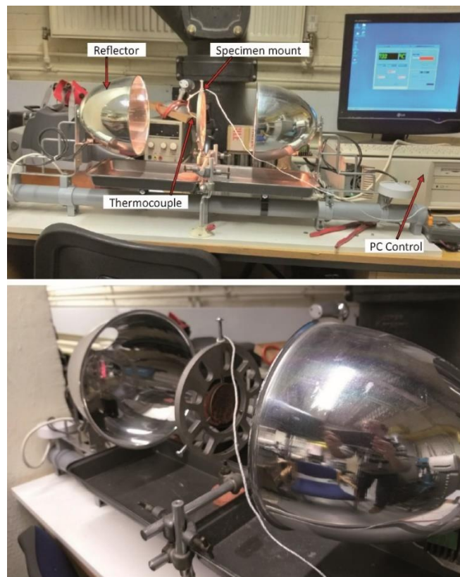
Figure 6.15: The thermal cycler apparatus created by Adam Wocjik with a ceramic disc specimen mounted.
