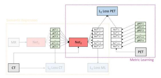
**Figure 6.4:** Purple dashed box: imitation network. A second CNN (*Net*<sub>2</sub>), HighRes3DNet, with pseudo CTs that were generated in stage one and corresponding CTs as input predicts the residuals between PET reconstructed with true CT-derived  $\mu$ -map and pseudo PET reconstructed with pseudo CT as  $\mu$ -map by minimizing  $\mathcal{L}_2$ -loss PET. Thus, this network imitates the PET reconstruction process.
