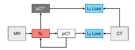
Figure 3.5: Recursive network architecture for pseudo CT synthesis. MR images are fed into a network  $N_u$  and an initial pseudo CT (pCT) is synthesized by minimizing an  $\mathcal{L}_2$ -loss (here: RMSE) between pCT and real CT. The pCT is then fed back into the same network in order to synthesize an improved version pCT\*, also by minimizing another  $\mathcal{L}_2$ -loss between pCT\* and real CT.
