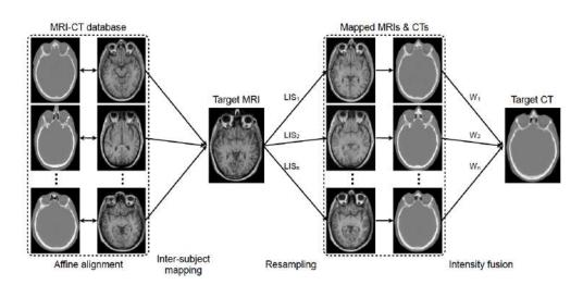
Figure 3.8: CT synthesis from a CT-MR database. All MRs within the database are mapped to the target MR before corresponding CTs are mapped to the target using the same transformation. A local image similarity measure (LIS) between the mapped and target MR images is then converted into weights to generate the synthetic CT (Burgos et al. 2014).
