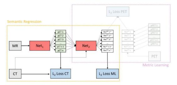
**Figure 6.5:** Final training stage: the first network is retrained with a combination of the CT  $\mathcal{L}_2$ -loss from stage one, and the proposed metric loss from stage two in equal proportions. The combined loss allows the network to minimize both the CT residual and the pseudo PET reconstruction error at the same time
