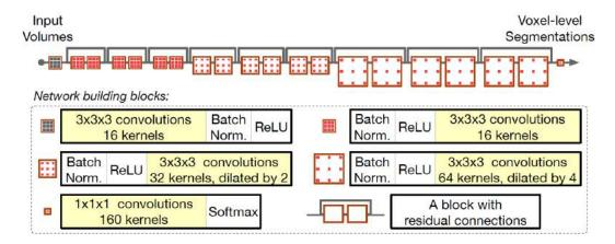
**Figure 3.2:** Original HighRes3DNet architecture from Li et al. (2017). Two crucial building blocks of this network are a) dilated convolutions with gradually increasing dilation factors in order to capture features at multiple scales and b) residual connections enabling identity mapping such that features from different scales can be connected. The network ensures that the spatial resolution of the input image is kept the same throughout the network.
