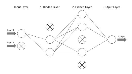
**Figure 5.5:** Dropout. During training time, random weights of the network are voided in order to avoid overfitting. At each training iteration, a different set of weights is dropped out. Crossed nodes have been dropped out, thus set to 0.
