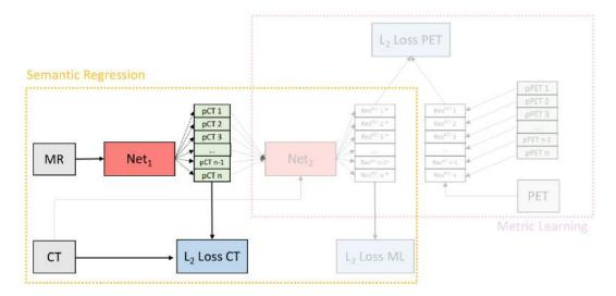
**Figure 6.3:** Yellow solid box: semantic regression. A first CNN (*Net*<sub>1</sub>), here HighRes3DNet, with MR images as inputs predicts multiple valid pseudo CT realizations by minimizing a combination of the  $\mathcal{L}_2$ -loss between true CT and pseudo CT ( $\mathcal{L}_2$ -loss CT).
