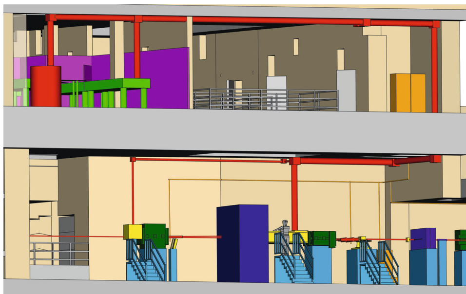
Fig. 100 CAD drawing of the XS1 access shaft building, including the LUXE experiment, zoomed on the laser transport pipe from the clean-room to the interaction point. The ICS set-up is also shown. The building is shown in beige and grey, while the different experimental elements are shown coloured
