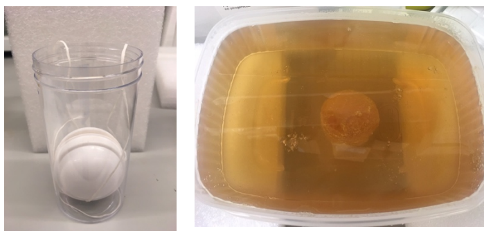
Figure 6. Creation of a radiopaque bead phantom. A: Agar filled sponge placed within a circular shell in order to create a 4 cm tumour B: 4 cm tumour placed within a box filled with liquid agar.
