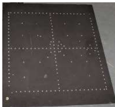
Figure 3.20: Glass plate and a network of images of it captured from different angles by one RedLake camera. These data provide a baseline calibration for each of the cameras and a quantification of the target image measurement capability.
