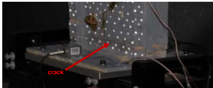
Figure 5.3.3: propagation of the crack – exp 5
