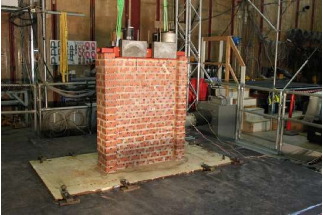
Figure App. III – 8: First large-wall specimen positioned on the shaking table along with the loadings fixed at the top of the large wall with the use of the stainless-steel loading case and the appropriate steel rods, at the University of Bristol
