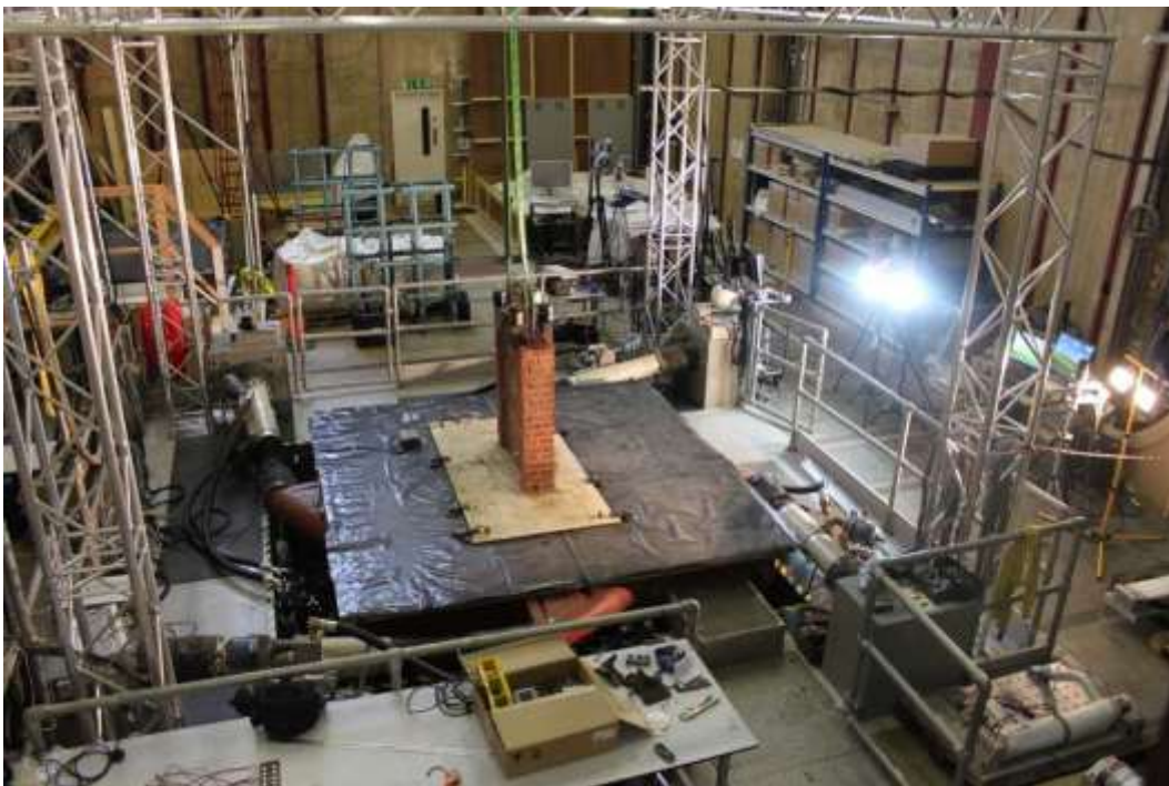
Figure App. III – 9: First large-wall specimen positioned on the shaking table along with the loadings; head-lights, cameras and computers placed on a desk opposite to the shaking table, at the University of Bristol
