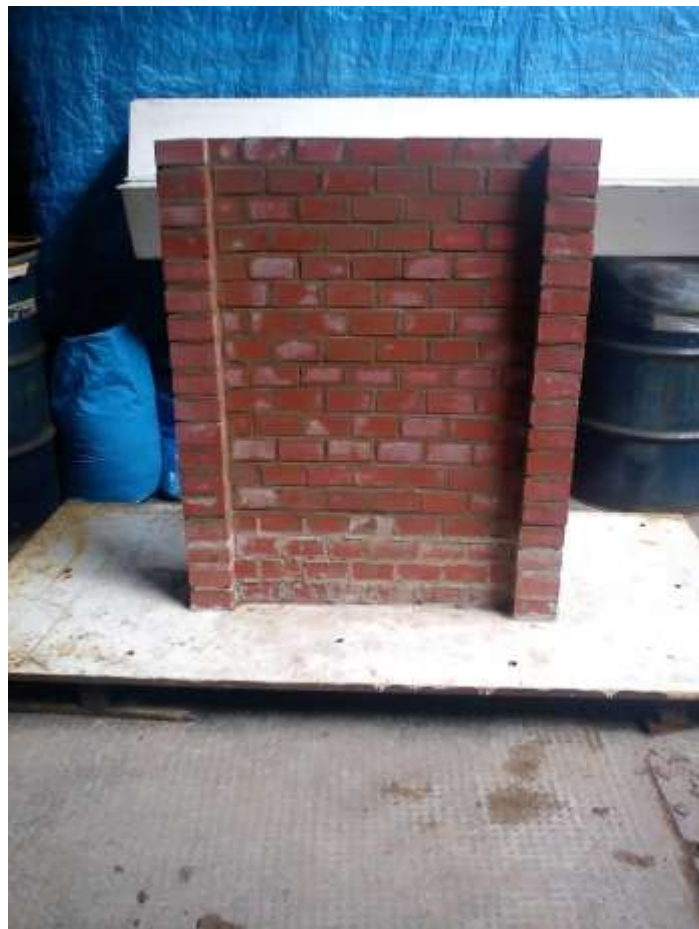
Figure App. III – 11: Front face of the large-wall specimens at the laboratory yard of the University of Bristol
