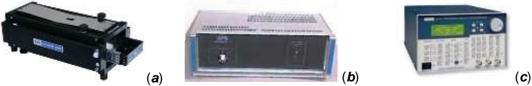
Figure 3.7: (a) Small Shaking Table; (b) Amplifier; (c) Function/Signal Generator (Shaking Table Laboratory Manual)
