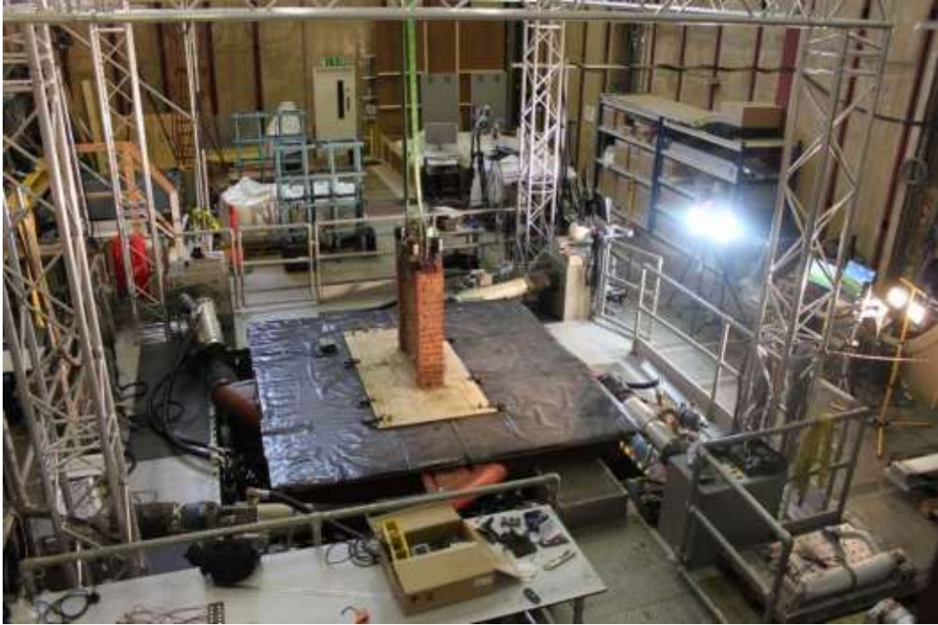
Figure 3.18: Large-wall specimen positioned on the large shaking table along with the loadings; headlights, cameras and computers placed on a desk opposite to the shaking table, at the University of Bristol
