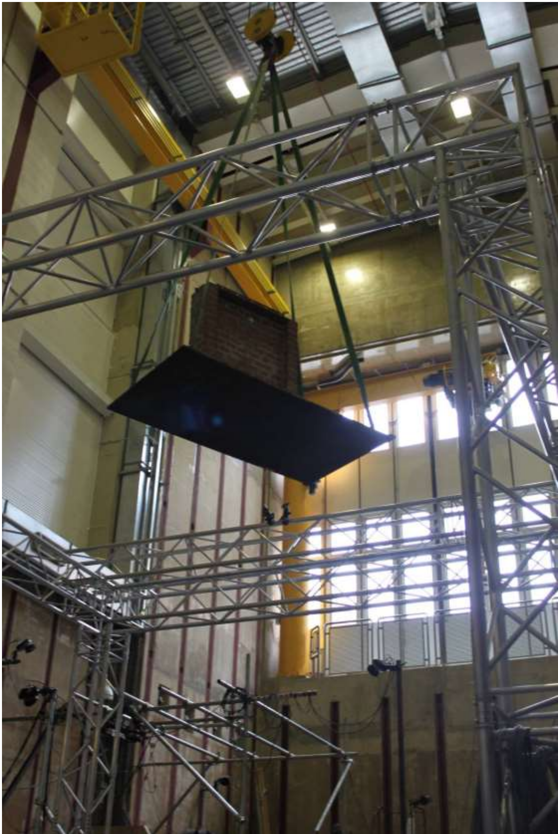
Figure App. III – 6: First large-wall specimen during its positioning on the shaking table with the use of the laboratory's crane, at the University of Bristol
