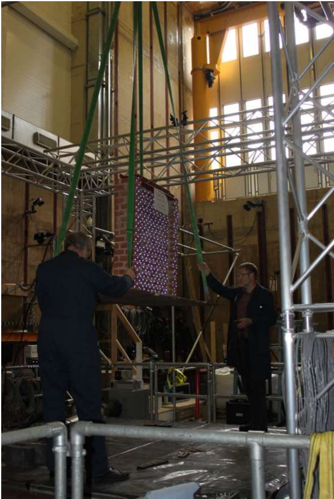
Figure App. III – 7: First large-wall specimen during its positioning on the shaking table with the use of the laboratory's crane being driven by the two technicians, at the University of Bristol
