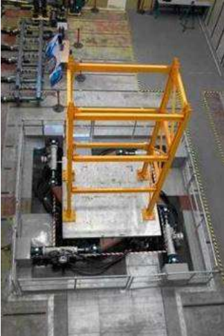
Figure 3.8: Large Shaking Table (University of Bristol web page)
