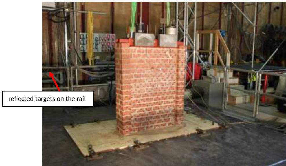
Figure 3.17: Large-wall specimen positioned on the large shaking table along with the loadings fixed at the top of the large wall with the use of the stainless-steel loading case and the appropriate steel rods, at the University of Bristol
