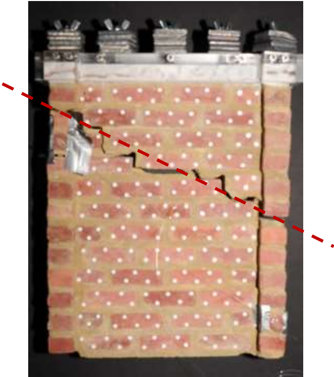
Figure 4.4: post-experimental phase of the tested wall – exp 1
