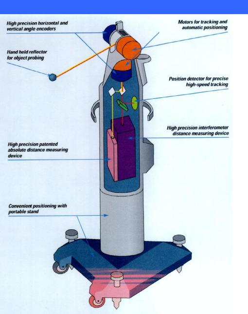
Laser interferometer accuracy ~ 1 ppm,
