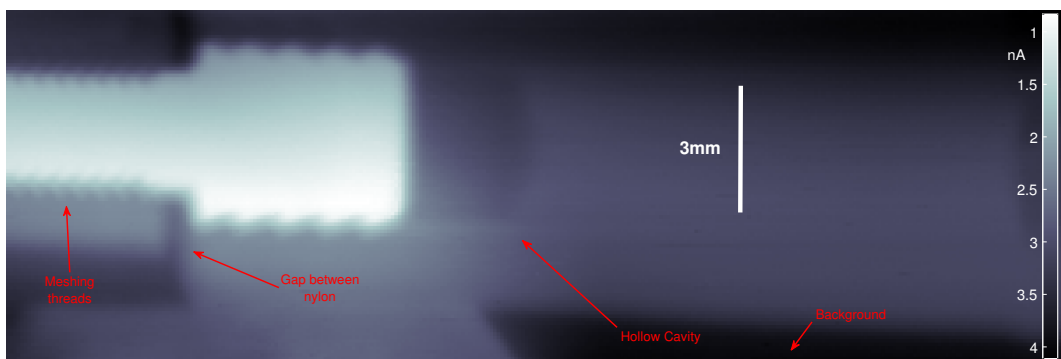
Figure 6.31: An X-ray image of nylon nuts joined by a brass screw, with a translation step of 100\ \mu\text{m} , and X-ray energy at 45 kVp and 10 mA
