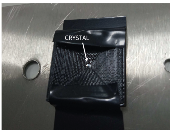
Figure 3.3: 3D printed sample holder for UV-Vis spectroscopy with crystal displayed at the centre.
