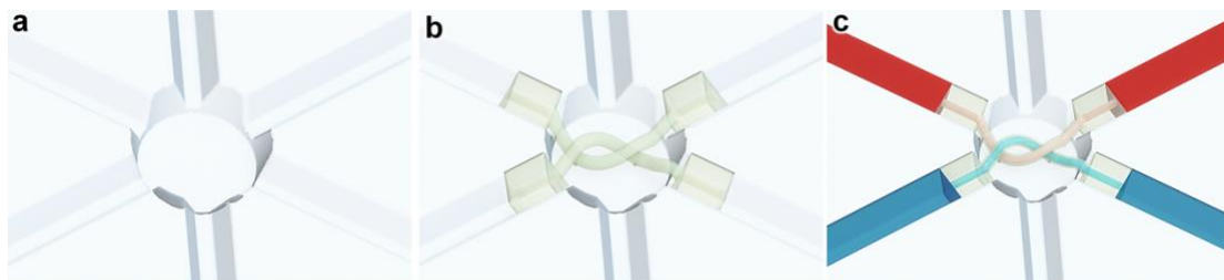
Figure 2.10: Conceptual illustrations of the: (a) empty COP-COP microchannel, (b) isDLW -printed microvessel structures, and (c) independent loading of distinct fluorescently labelled fluids.
