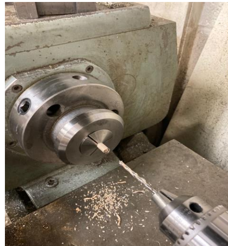
Fig. 3.1. Sample drilling via lathe machinery.
