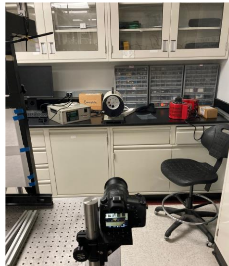
Fig. 2.1. Experimental setup of the camera calibration to the blackbody emitter.
