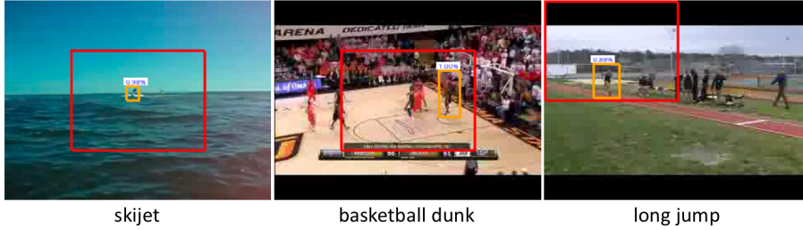
Figure 5.12: Examples of the small scale action detection by our approach. Red boxes indicate the initial proposals and orange ones the detection outputs.
