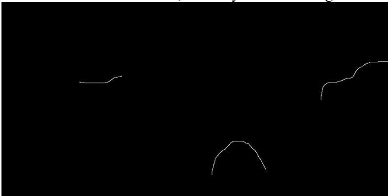
Tx3 Mask of the traced cracks after manual tracing
