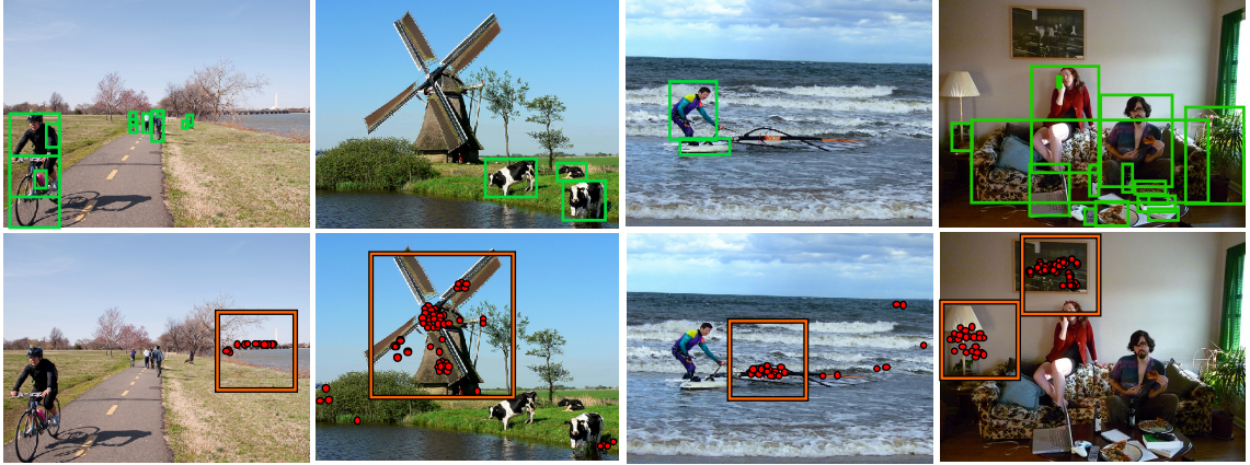
Figure 2.2: SNIPER negative chip selection. First row: the image and the ground-truth boxes. Bottom row: negative proposals not covered in positive chips (represented by red circles located at the center of each proposal for the clarity) and the generated negative chips based on the proposals (represented by orange rectangles).
