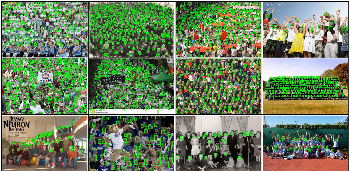
Figure 5.9: Qualitative results on the validation set of the WIDER dataset. Green rectangles show the detection and brightness encodes the detection confidence.
