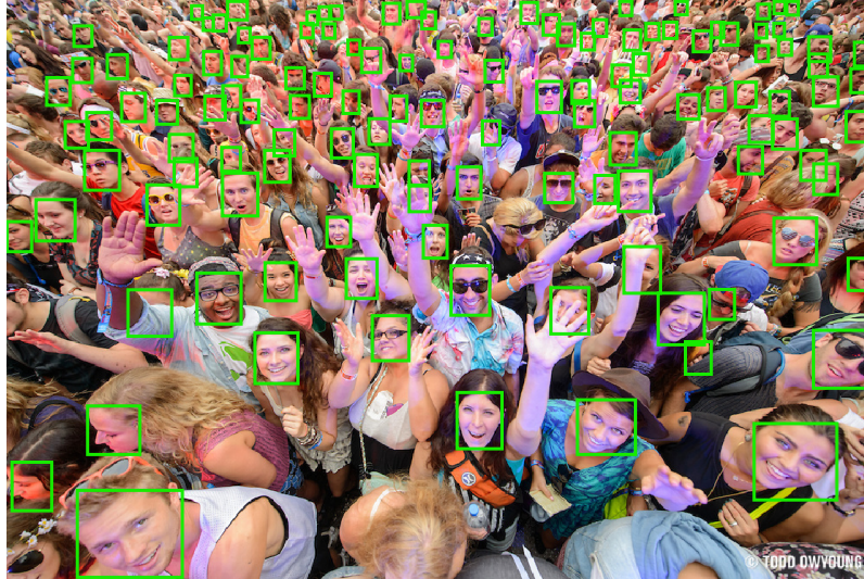
Figure 4.1: SSH detects various face sizes in a single CNN forward pass and without employing an image pyramid in \sim 0.1 second for an image with size 800 \times 1200 on a GPU.
