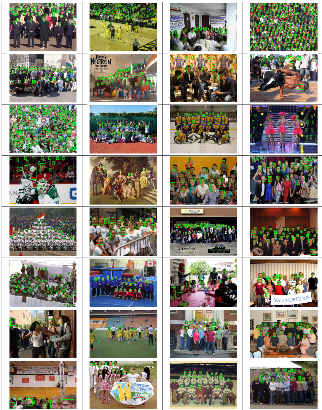
Figure 4.8: Qualitative results of SSH on the validation set of the WIDER dataset. Green and blue represent a classification score of 1.0 and 0.5 respectively.
