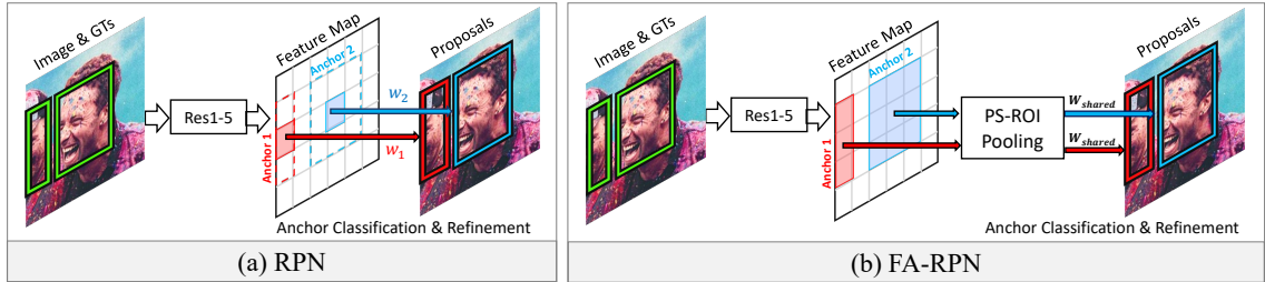
Figure 5.2: We highlight the major differences between RPN (a) and FA-RPN (b) proposals. RPN performs classification on a single pixel in the high-dimensional feature-map and uses different weights for classifying anchor-boxes of different sizes/aspect ratios. FA-RPN proposals, on the other hand, pool features from multiple bins in the image and share weights across objects of different sizes and aspect ratios.
