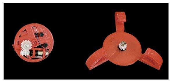
Figure 3.9: The turntable mechanism. When the bot makes contact with the copper pads on top and sends a signal through the motor driver, the rotor rotates around the base, which also rotates the bot.
