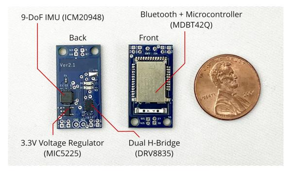
Figure 3.4: Custom PCB designed to maintain a small device footprint.
