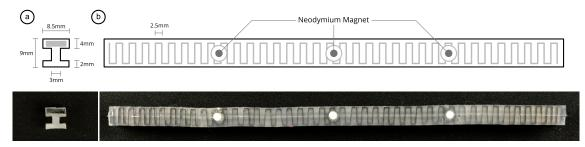
Figure 3.5: Meta-material track design. a) Cross-section of the track. b) Top view of the track with embedded magnets and a live-hinge pattern of the inlay.
