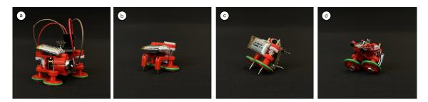
Figure 3.1: The different design iterations of Calico. a) The proof-of-concept with 4 wheels and 2 Pololu Micro Metal Gearmotors. b) Switching to a smaller motor with a different gear assembly. The overhangs would easily get caught on wrinkles in the clothing. c) Switching to a copper shaft to avoid the overhangs but still create electrical contact with the turntable. d) Switching to dual motor drive and magnets with copper plates to increase the speed and the climbing capacity.
