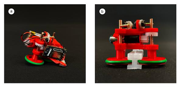
Figure 3.2: a) The Calico bot. b) The latching mechanism used by the Calico bot to move along the track.
