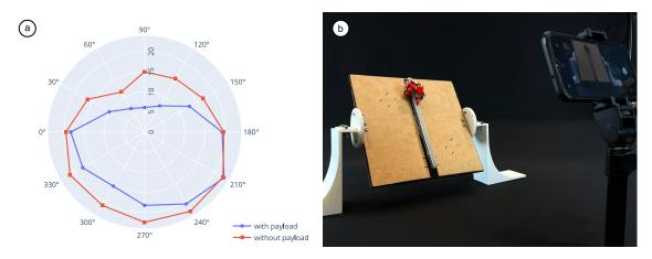
Figure 4.1: a) Speed in  $cms^{-1}$  with and without a payload (20gm) plotted against approach angle. b) Test setup used to test the speed with and without a payload.
