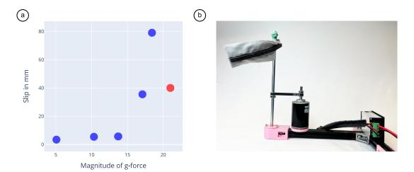
Figure 4.3: Testing the slip of the device when subjected to different g-forces. a) Scatter plot showing the slip vs the g-force encountered. At 21g (marked in red), the wheels broke through the inlay instead of slipping along the groove in the track. b) Test setup used to run the experiment.
