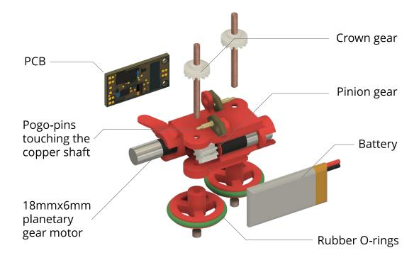
Figure 3.3: An exploded view of Calico
