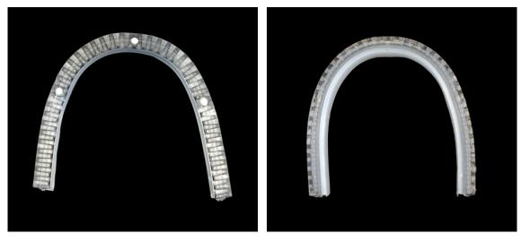
Figure 3.6: Due to the live-hinge design, the track can be flexed in all directions while still restricting the degree of freedom to keep the wheels of the bot in the crevice.
