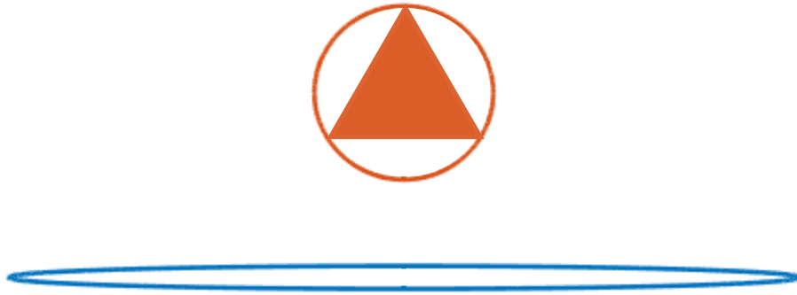
Figure 102: Cross sections of equivalent flow area and hydraulic diameter, but the first with a triangular insert, the second without insert
