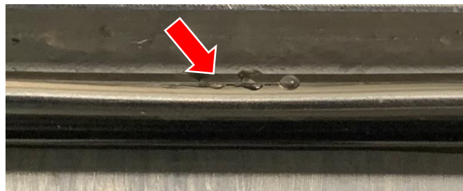
Figure 42: Longitudinal crack that leads to heat transfer fluid leakage
