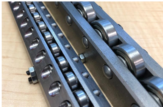
Figure 121: Photo of the two rails used to constrain the single tube.
