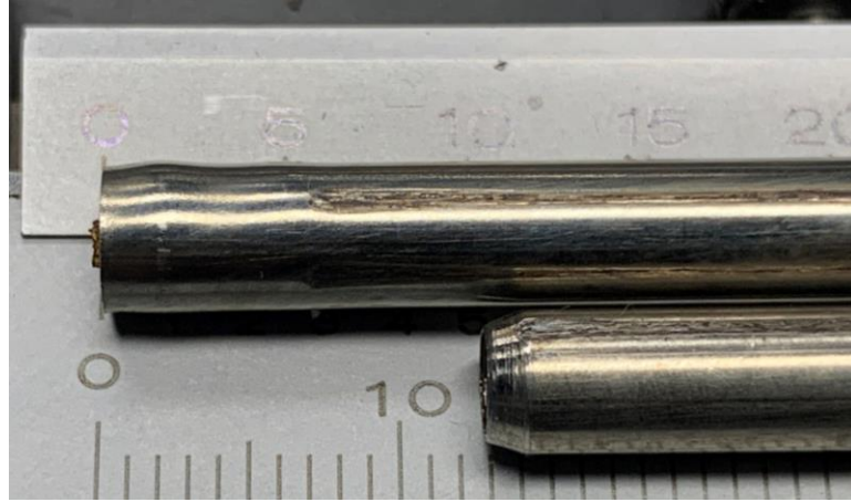
Figure 40: Distance between end of Ni-Ti tubes and support stainless steel tubes (ruler units: mm).
