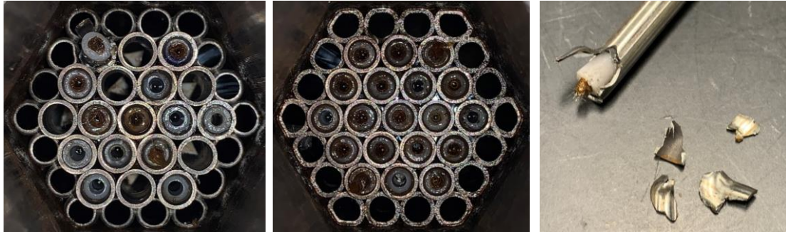
Figure 41: Broken Ni-Ti tube and deformation in stainless steel tubes
