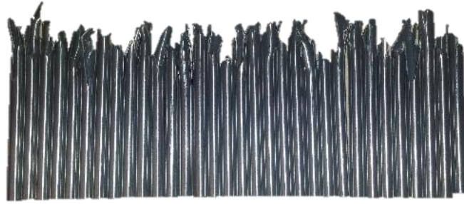
Figure 39: Photo of Ni-Ti tubes catastrophic failure (internal report by Qian)
