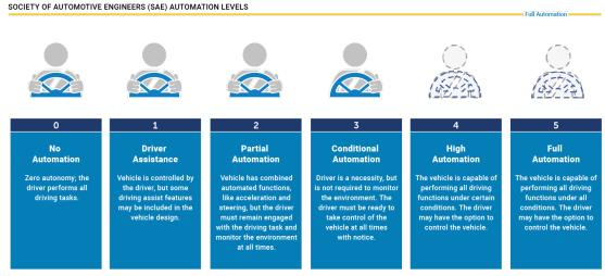
Figure 3.4: Autonomation Levels. (Source: Society of Automotive Engineers)
