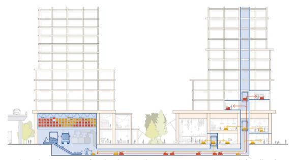
Figure 3.7: Logistics Hub and underground connection concept. (Source: Sidewalk Labs, Toronto Tomorrow, 2019)
