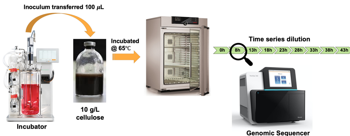
Figure 3. Graphical representation of Biogas reactor Dataset. A 100 µl inoculum was collected from a lab-scale biogas reactor incubated at 55°C and transferred to an anaerobic flask containing 10 g/L of cellulose. Triplicate mRNA samples were taken in a time series from 0 to 43 hours after inoculation. Metagenomic and metaproteomic sequencing was performed for all time points. For this tutorial we used one of the triplicates (T1A) in the 8 hours' time point.
