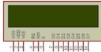
Gambar 2. Diagram pin LCD tipe HD44780 [3]
