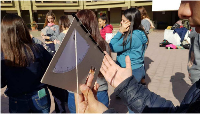
Figure 3. A student using a quadrant made of simple materials, to measure the Sun's altitude.
